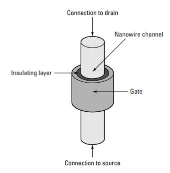
Using a nanowire as the channel allows you to completely wrap the gate around the channel. This should allow the voltage applied to the gate to have even more control over the channel than when using the finFET (refer to Figure 6-2). This vertical structure also saves space, allowing a higher density of transistors on a chip. Millions or billions of vertical nanowires could be grown on a substrate, like a dense but tiny forest.
